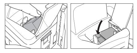
**7** Make sure that the ink cartridge lock lever locks the ink cartridge into the correct position.
